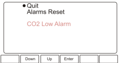
Figure 11. Active Alarms menu
