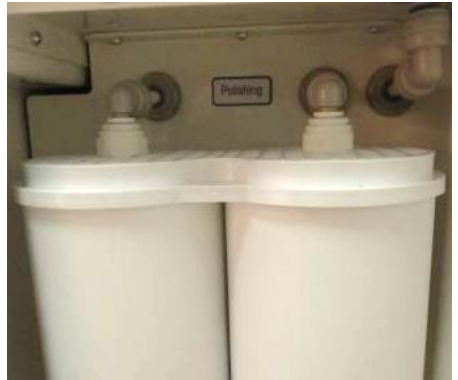
Figure 14. Fitting the module inside the unit.
