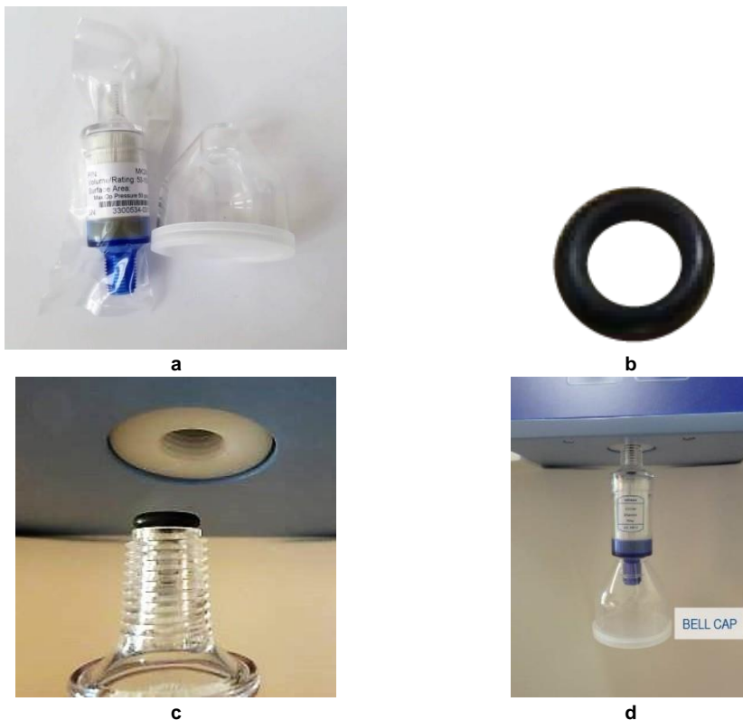
Figure 20. 0.22 \mu\text{m} filter dispenser installation.
