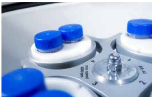
Bucket rotor BR-4U with BA-2/50 adapter
